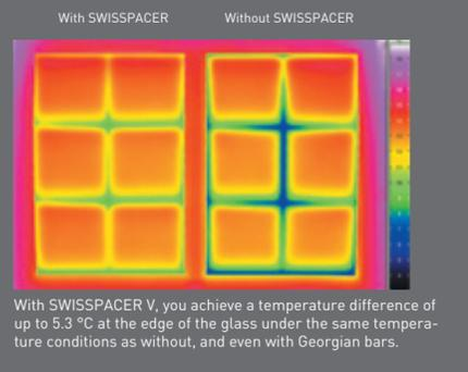
With SWISSPACER V, you achieve a temperature difference of up to 5.3 °C at the edge of the glass under the same temperature conditions as without, and even with Georgian bars.
