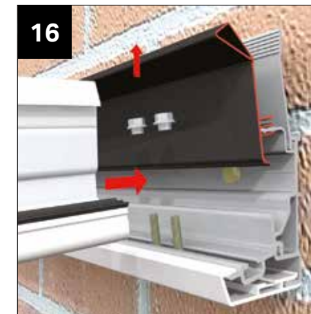
Ensure the rain baffle upper leg is lifted prior to placing the glazing bars that fit to the ridge body sides.
