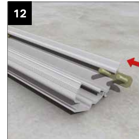
Make sure the appropriate number of roofing bolts are located in the bolt slot of the wall plate before finally fixing the wall plate to the wall.
