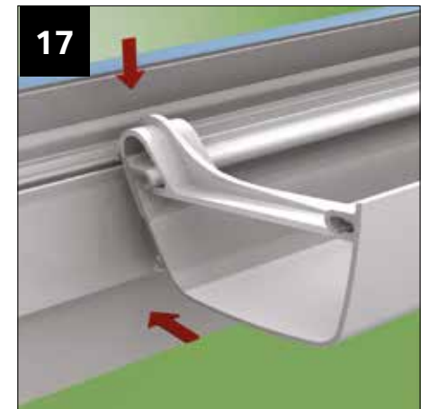
Locate the gutter brackets, stop end and stop end outlet and lift into position on the external fascia. Push down to locate the lower leg of the bracket. Assemble the rain water pipe, attach to the gutter and screw to the frame.
